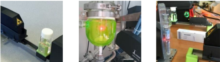
Measurement in a custom container – no batching In situ monitoring in a double jacket glass reactor Analysis of injectable vaccine in a prefilled syringe
